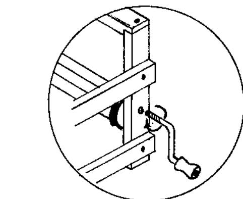
Insert shaft of back beam MB-14 in hole of left post MB-8. Put the wire circle around the plain wheel MF-2 for friction brake and screw the crank MA-9 in beam.
