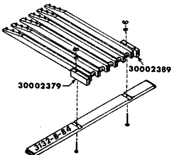
Insert blocks 30002389 and 30002379 in treadle shaft.
