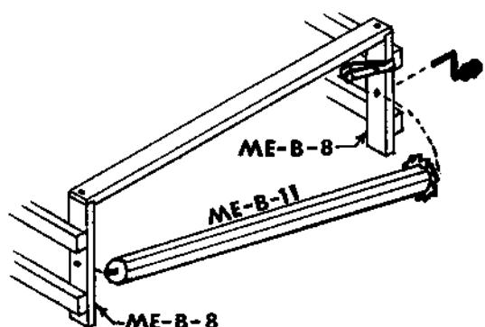
Insert shaft of cloth beam MB-11 in hole of left post MB-8. Lift the ratchet dogs and screw the crank MA-9 in beam.
