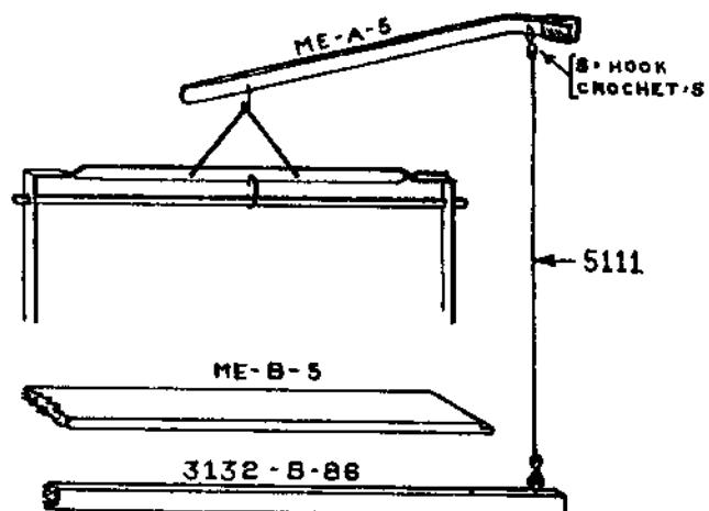
Place the S hook of cord 5111 in hole on lever ME-A-5 and insert the other end of cord in lam's hook. Close the S shaped hook, so it stays in place.
