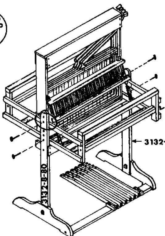
Fix the lams in the bracket 3132-B-85 with a machine bolt  $\frac{1}{4}$ " x 3" and square nut. Fix the lams bracket 3132-B-85 with a carriage bolt 5/16" x 2" and square nut in the last hole of left upright 3132-B-80.
