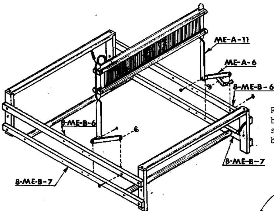
Replace the batten and screw brackets MA-6 and batten swords MA-11 to the cross bars 8-MB-6 and 8-MB-7.
