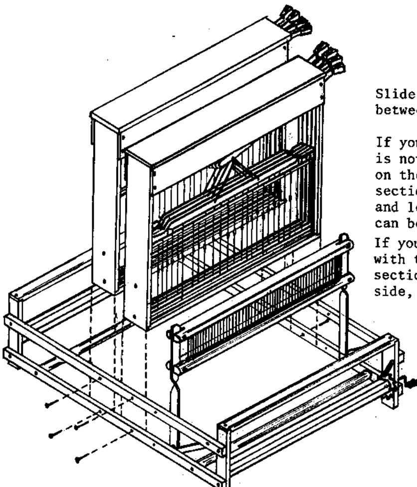
Slide the two 4-harness sections between the cross bars and screw.
