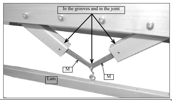
The friction between the metal pieces M, the spring pin of the jacks and the S Hook may produce unpleasant noise that can be eliminated by spraying silicone spray in the indicated area.
