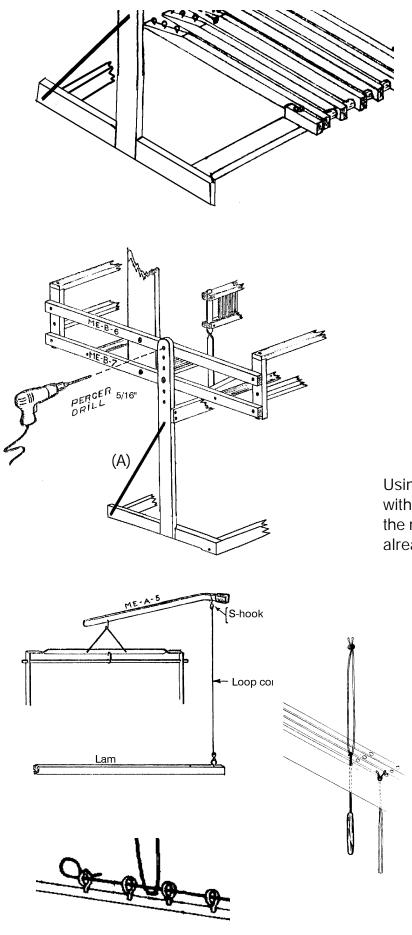
Screw the Upright post to the base using the 4 Carriage bolt  $\frac{1}{4}$ " x 1 $\frac{3}{4}$ ", 4 washers  $\frac{1}{4}$ " and 4 square nuts  $\frac{1}{4}$ "
