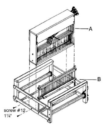
After unpacking the loom, unfold the base and put the two little metal hooks (at the front side) in position (over the screws) and screw them in slightly so they hold in place. Take off the machine screws which are at the end of the beams and attach the crank to the right hand side by turning it. Because the metal of the crank is plated, it may be little difficult to attach the crank but take your time, it is the right size.
