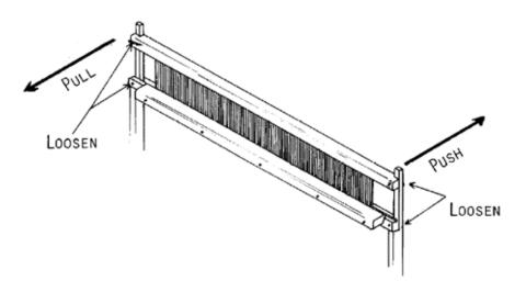
The beater has been adjusted at the factory before shipping. If the batten doesn't touch the two bumpers equally, loosen the bolts of the batten sley and batten handtree and exert pressure on the batten centering it in its proper place. Tighten the bolts again while keeping pressure on the batten.
