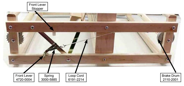
The length of the loop cord has been marked (black mark) and tested before shipping. After some time, the loop cord may stretch. You will then have to readjust the tension by changing the loop on the cord. When the front lever is release (to the front lever stopper), the brake circle (around the brake drum) should be loose enought to be able to turn the back beam.
