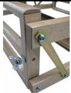
This system will eliminate excessive warp yarn advance when releasing the brake system at cloth take-up. This friction system is adjustable and have to be released when winding the warp on. Just screw the wing nut with nylon bolt to the left back post. Screw in to increase the friction or unscrew it to release.
