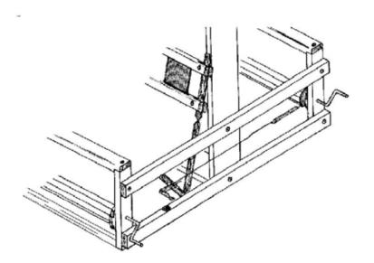
For an 8s loom, install the shaft frame section with beater bumber in the front (lever at the right side of the loom). Install the second shaft frame section levers at the left side of the loom.
