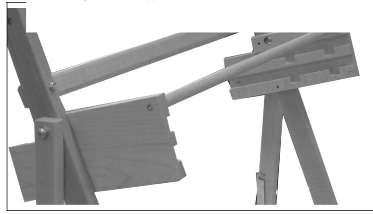
Install the middle slide post useing the 2, #8, 1" flat headed screws. Do not overtighten. If the reeds do not slide properly, loosen the slide post slightly.
