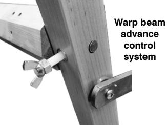
This system will eliminate excessive warp yarn advance when releasing the brake system at cloth take-up. This friction system is adjustable and have to be released when winding the warp on.
