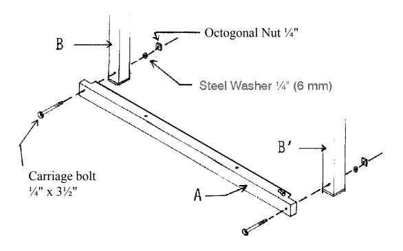
Using two  $\frac{1}{4}$ " x  $3\frac{1}{2}$ " (6 mm x 89mm) carriage bolts, two  $\frac{1}{4}$ " (6mm) steel washer and two octogonal nuts  $\frac{1}{4}$ ", attach the front cross-member A to front posts B right and left.
