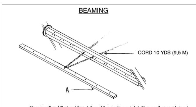
Thread the 10 yard (9 m) cord through the middle hole of beam stick A. Then pass the two ends (equal in length) of this cord through the middle holes of the warp beam.
