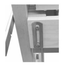
After the Jack box is installed, remove the two screws at the back right corner of the jack box, install the metal protection plate and reinstall the screws to hold it in place. This plate protects the wood from damage by the brake lever when the back beam of the loom is folded in.
