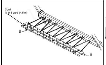
Cut the 5-yard (4.5 m) cord in half. One half of this cord laces beam stick A to warp rod B
