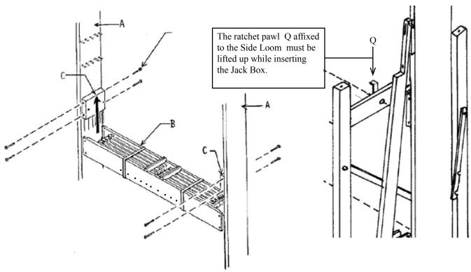
Slide jack box B along the middle posts A, from bottom to top, and affix it to blocks C using eight 1½" (40 mm) round-headed screws no. 12.
