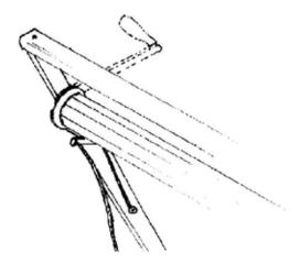
Using two 2" round-headed screws no 14, affix the breast back beam to the back posts.
