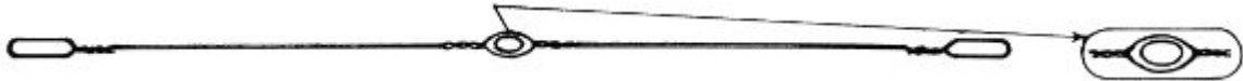
Inserted eye heddles: wire heddles with special oval shaped eye. Heddles do not catch on each other. They slide easily on heddle support. Warp threads ride through eye smoothly.
