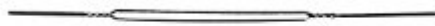
LONG EYE HEDDLES: the inside dimension of the eye is 2" x 3/32" (50 mm x 3 mm)
