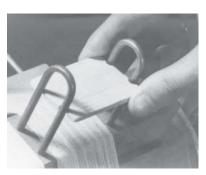
Useful when beaming long warps. They are placed in each section every 5 or 10 yards (meters) to prevent uneven build-up of threads and keep uniform tension in the warp. They all have to be placed in the same turn
