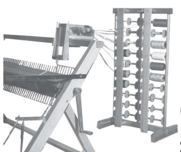
This system consists of 4 rake-like pieces that are attached to the plain beam on the loom or onto the double warp beam. It allows warp beaming 1" or 2" wide (25 mm or
