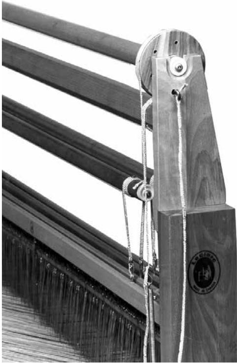
A shed regulator is an attachment for counter-balanced looms such as the Leclerc "Mira" or "Fanny". It allows a perfect shed on any tie-up. Used to regulate the height at which the shed opens for unbalanced tie-ups, such as Bronson, Waffle, Double Weave, circular weave, etc.
