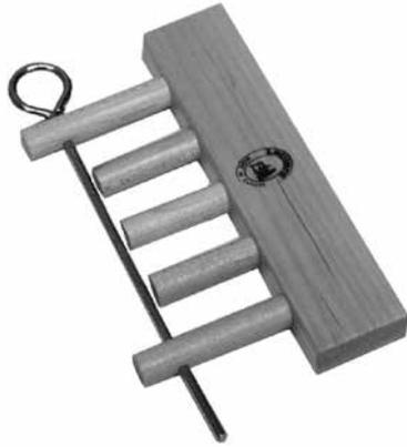
Used on counter-balanced and counter-march looms to keep shafts at same level and distance while threading.
