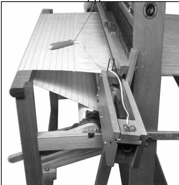
The flying shuttle is a beater with shuttle boxes at each end. A hammer in the shuttle box, put in motion by a cord and handle, strikes the shuttle, and sends it through the shed without the weaver touching it. Flying Shuttles are useful in weaving studios where long yardages are made. Time is saved in weaving wide fabrics where it is difficult to throw and catch the shuttle.
